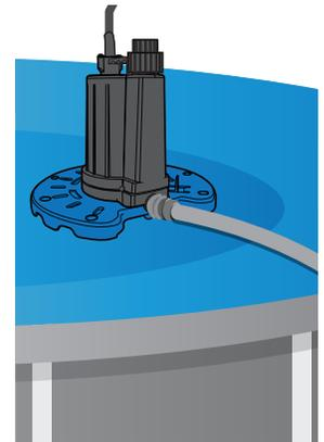
5. Plug the pump into a properly grounded, ground fault circuit interrupter (GFCI) 115 V outlet. For safety, the pump should always be electrically grounded to a suitable electrical ground, such as a grounded water pipe, properly grounded metallic raceway, or ground wire system.
