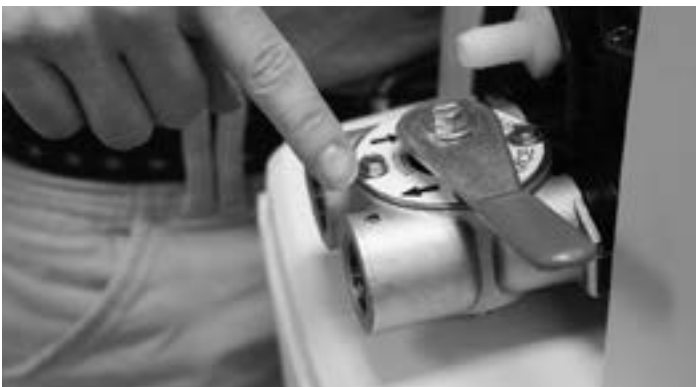
10. Check inlet and outlet for correct water flow, matching arrows on valve head and on by-pass valve (especially if replacing an existing unit). CAUTION: Install in directions of arrows.
