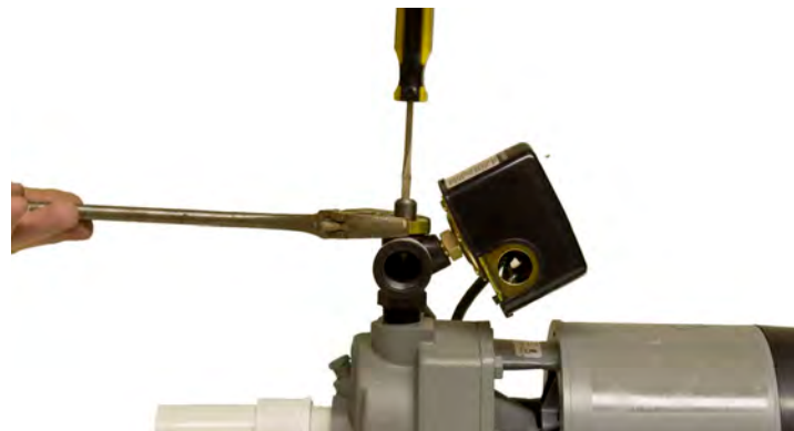
5. With pump operating at high pressure, open two or more faucets and slowly unscrew the flow control screw until maximum flow is obtained. This steady pressure will be minimum operating pressure and should agree with the pressure shown below. The flow control screw diverts the proper amount of water to operate the ejector. (Fig. 5)
