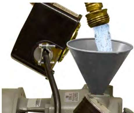
2. Fill pump cavity with water until full and replace priming plug. (Fig. 2)
