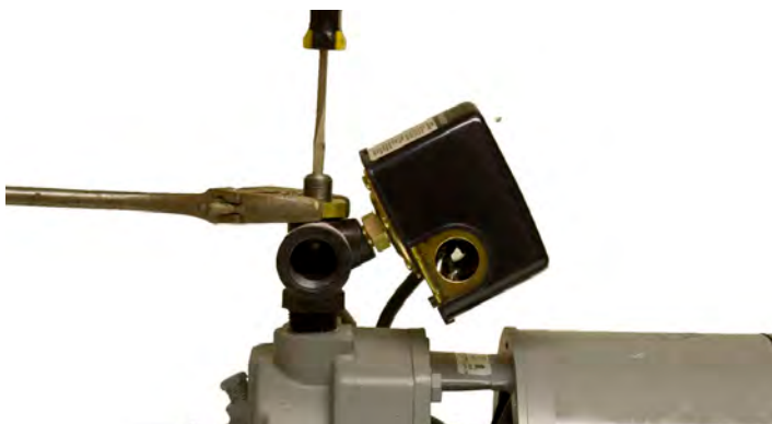
3. Tighten flow control screw completely by turning clockwise, then loosen two turns. Now start the pump. (Fig. 3)
