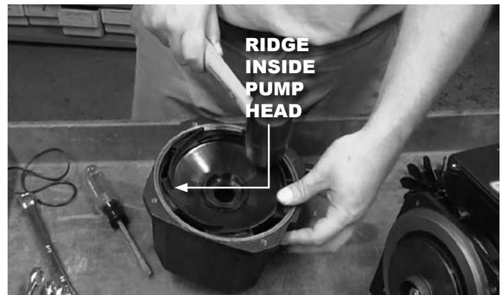
19. Reinstall the o-ring so it seats inside the ridge inside the pump body.
