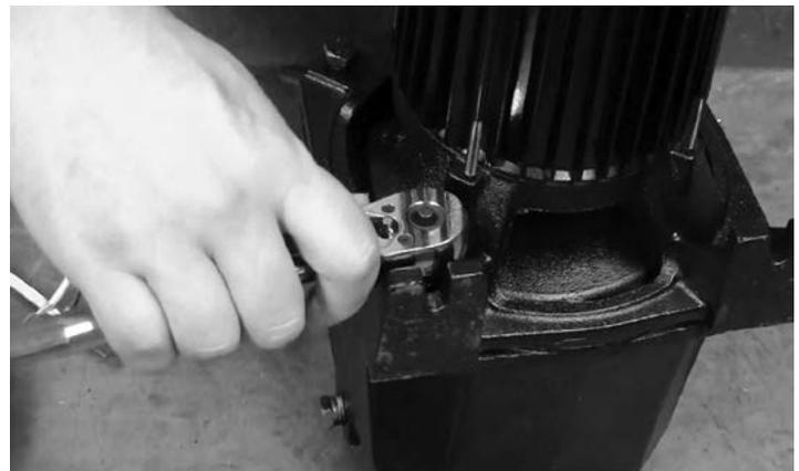
22. To reinstall the fan, find the flatted portion of the fan opening and the flatted portion of the shaft. Line those two up. Press the fan back in place and replace the motor cover.
