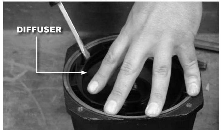
18. Discard the old diffuser, and install the new one from the repair kit. Alignment isn't required, but it may need a tap from a rubber mallet to seat back into the ridge inside the pump head.
