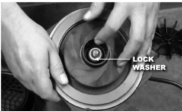
9. Once the lock washer is removed, slide the impeller off of the shaft.
