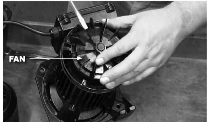
7. You will use a 14 mm socket or wrench to hold the shaft stationary while you remove the 17 mm nut from the other side of the pump.
