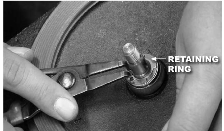
12. Remove the flat washer located under the retaining ring, and pry the seal off of the shaft with a flat screwdriver. Discard the old seal.
